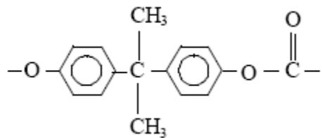
Although of low crystallinity it has unusually high impact resistance for a plastic and is used, for example, for crash helmets.
