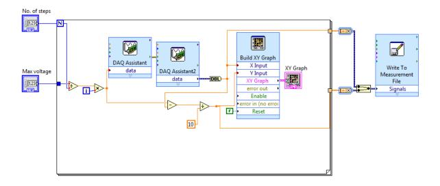
You can run your VI. The Max V generated by the DAQ is 5 V. Use at least 15 steps to obtain a smooth diode characteristic curve.
