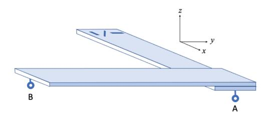
Figure 1: The cantilever beam with strain gauges, used for bending and torsion experiments
