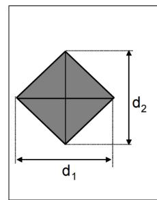
Hardness is defined as the pressure on the contact area of the indentation impression: For the 'Vickers' diamond pyramid profile the Vickers Hardness Number (HV or VHN) is given by:
