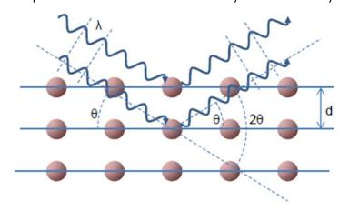
be an integer number (n) of wavelengths ( $\lambda$ ) for coherent diffraction. This can be written in terms of inter-planar spacing (d) and angle ( $\theta$ ) as Bragg's law:  $2d \sin \theta = n\lambda$  where n=1.
