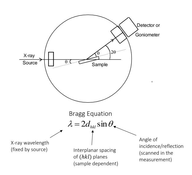
All X-ray goniometers will have a **background** number of counts even when no crystallographic planes are aligned at the Bragg angle. Any two diffractometers will show have different characteristic backgrounds, but they are usually only important for small grained-powder samples or those which have a low peak/background ratio for other reasons.
