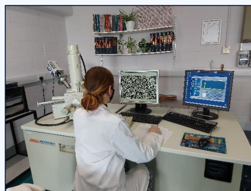
Using a Scanning Electron Microscope to investigate crystal structures and fracture surfaces during laboratory sessions
