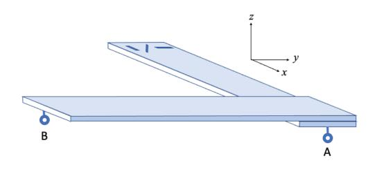
Figure 1: The cantilever beam with strain gauges, used for bending and torsion experiments
